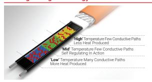
The simple 120 V Plug-n-Play system is ideal for residential and small commercial buildings and requires no specialist electrical knowledge. Simply fix to the pipe, insulate and plug into a ground-fault protected electrical outlet. It is that simple.
