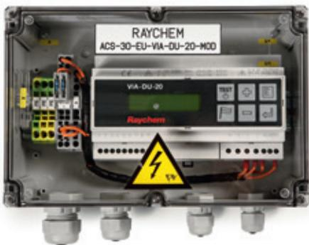
The RAYCHEM ACS-30-EU-VIA-DU-20 Module for the ACS-30 system provides smart sensor input for surface snow melting and de-icing applications. The module provides ground temperature and moisture sensing for the ACS-30 control system. The module can be positioned near to the heated area and is connected to the PCM module via a 3-wire cable. The module is provided with a 15m external ground temperature and moisture sensor to be positioned at the heated surface.
