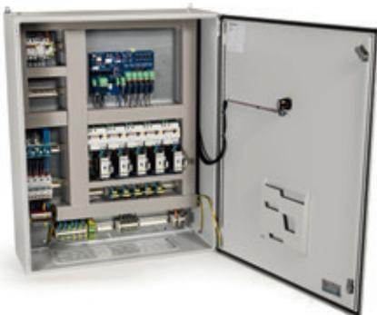
The ACS-30 PCMs provides power connection, with built-in electrical safety devices, line current sensing, alarming, switching (electromechanical relays) and RTD inputs for the heat-tracing circuits when used with the UIT. The ACS-30 PCM enclosure is rated IP54 to EN60439 and is approved for nonhazardous indoor or outdoor locations.
